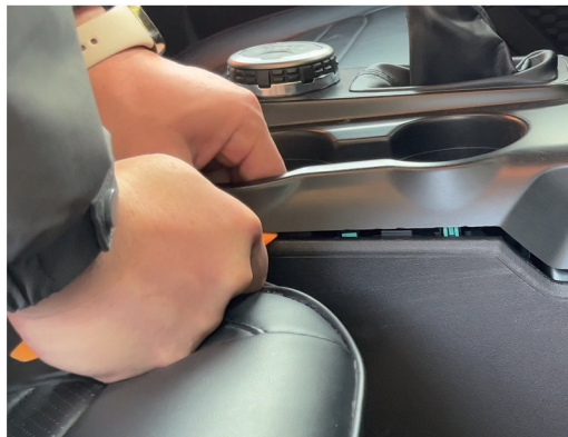
16 The back end pulls upward as you pry.
