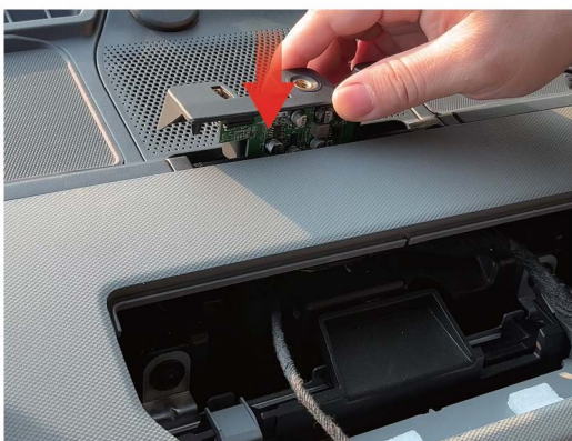
27 Pull the harness all the way through.
