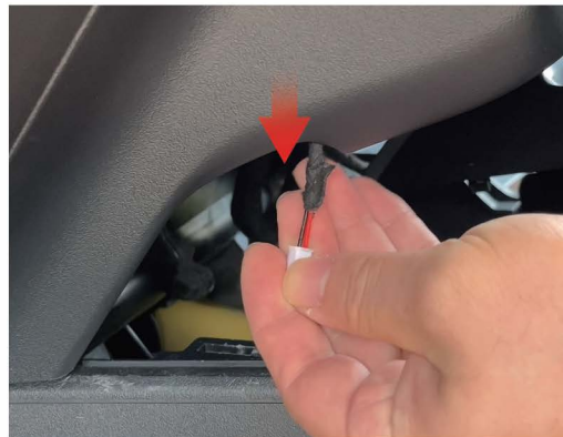
31 The harness may not pass through directly. You can reach in with your hand to and pull it downwards.
