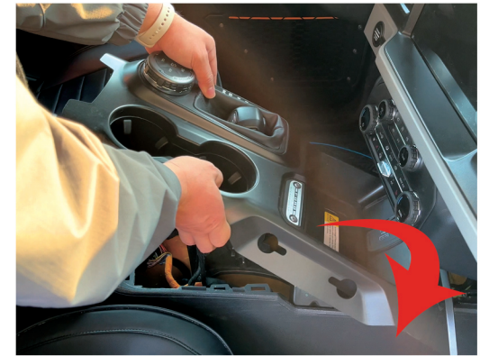
18 Lift up the central control panel and rotate it until you can see the socket in the next step.
