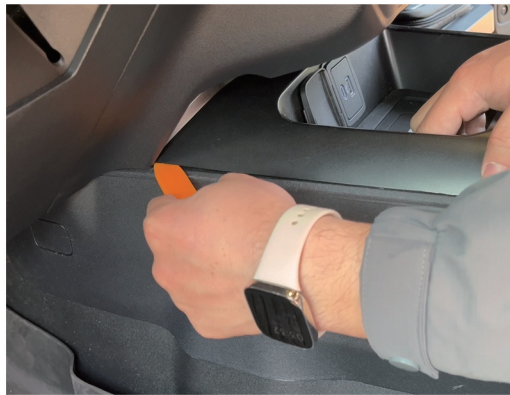
12 Use a pry bar to pry the center console through the front end gap.
