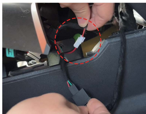
33 Plug the white small plug that has been passed through into the remaining white small socket.
