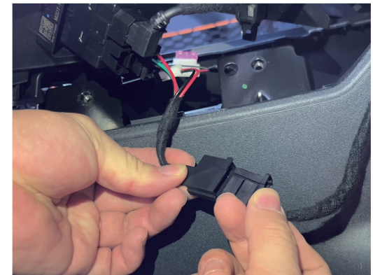
22 Find the plug end of the harness and insert it into the socket mentioned in step 19 (the original vehicle plug has been unplugged).
