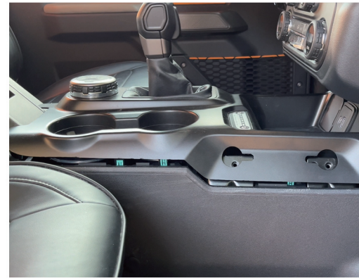
17 The entire center control is then pried up all the way.
