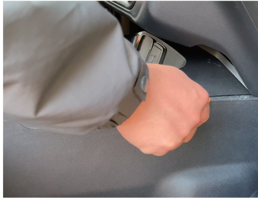
14 Go to the other side and start prying at the clips.
